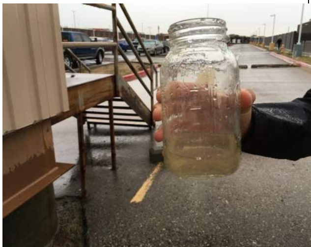
Outfall D1 – Stormwater sample collected from manhole
